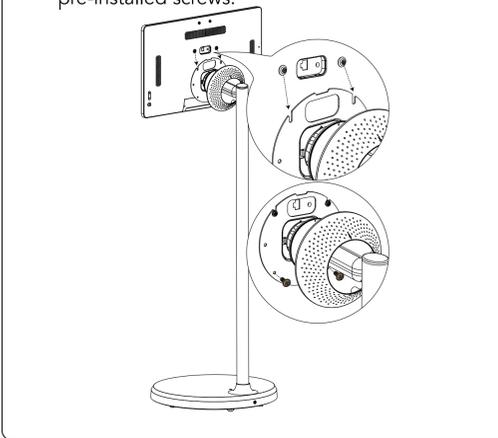
**08** Check whether all four screws are locked in place, and then insert the bracket power cord into the display base.
