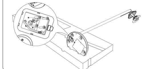
**05** Insert the bracket power cord into the charging board base and then snap on the cover.
