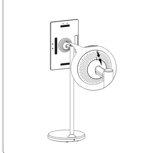
**10** Align the camera hole with the display hole, lock the two (PM3\*5) screws in place, remove the dust cover, and then plug the connection cable into the blue USB3.0 port of the display. The installation is complete.
