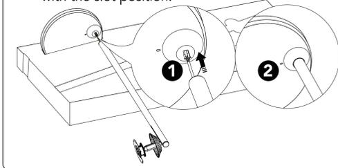
**04** Lock the four screws (A bag BM3\*16) on the base (tip: fix the diagonal position first).
