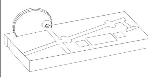
**03** Thread the bracket power cord through the base and install the bracket on the base by aligning it with the slot position.
