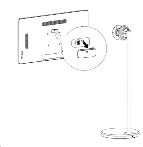
**07** Align the two pre-installed screws on the VESA of the display with the U-shaped hole on the bracket, slide them in to fix them, lock the remaining two screws (B bag PWM4\*6), and finally tighten the two pre-installed screws.
